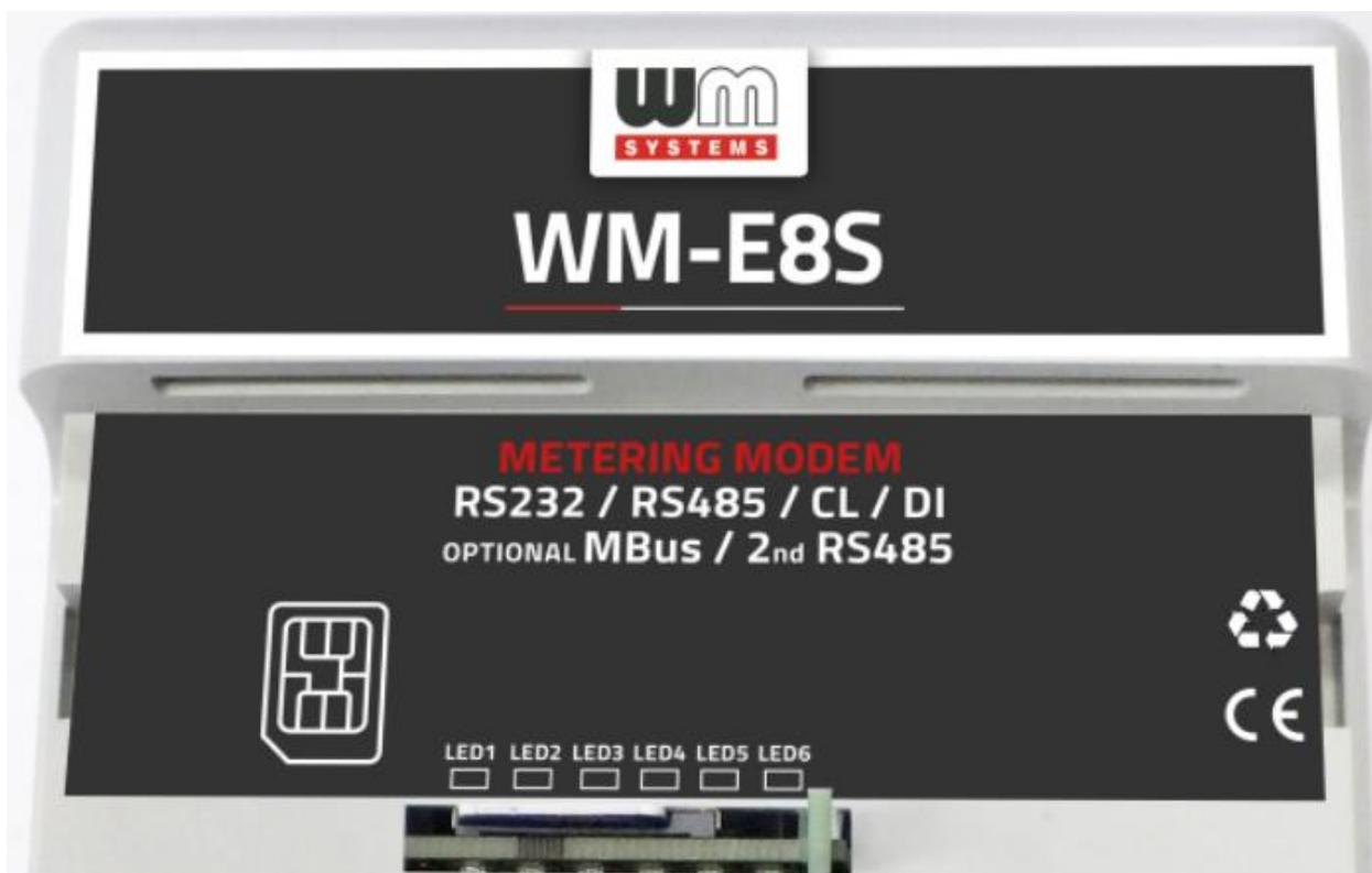
At the first power-on - during charging of the supercapacitors - **LED 3** starts flashing quickly by **green**, while **LED 6** blinks once every 2 seconds by **green**.
