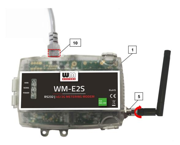
*Step #14:* Configure the modem with the WM-E Term<sup>®</sup> configuration software.
