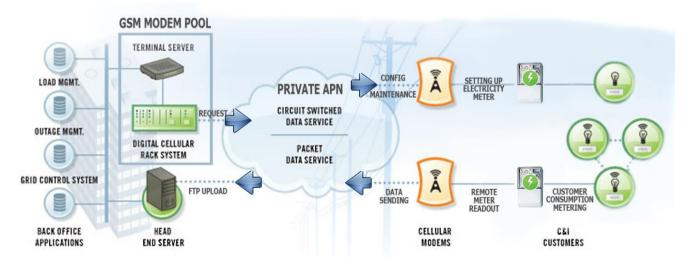
There is another option and meter data sending mode to initiate a remote readout automatically in pre-defined intervals. It is also possible to start the data sending in case of different events (e.g. removal of meter cover, incoming SMS message from the centre).
