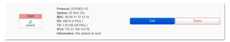
As you can see, the device is already connected to the mobile internet network and is currently active - **RX** (received data), **TX** (sent data) and **KB** (KBytes) are constantly increasing.
