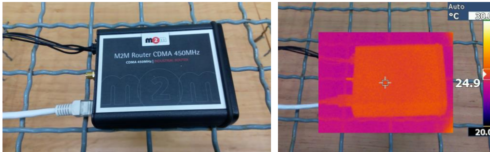
Figure 4. Test arrangement and thermal image of the device after the application of the reversed voltage
